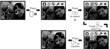
The Status LED flashes to indicate that the countdown is being performed, it flashes quicker and the camera beeps after 8 seconds. The long beep sounds indicates the picture is successfully taken. The self-timer turns off automatically after taking a picture.
